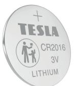
**DESCRIPTION:** Mercury Free Lithium Cell Battery, CR2016 / Non-Rechargeable **CHEMICAL SYSTEM:** Lithium Manganese Dioxide SHELF LIFE: 7 years **NOMINAL VOLTAGE:** 3 Volts **NOMINAL DIMENSIONS:** Ø 20 mm × 1.6 mm **APPLICATIONS:** Suitable for flashlights, car keys, watches, scanners etc. **STORAGE TEMPERATURE:** +10 °C to + 25 °C Should be stored in dry and cool place. **NOMINAL WEIGHT:**
